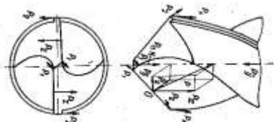
1- rasm. Parmalash jarayonida ta`sir etuvchi kuchlar sxemasi
