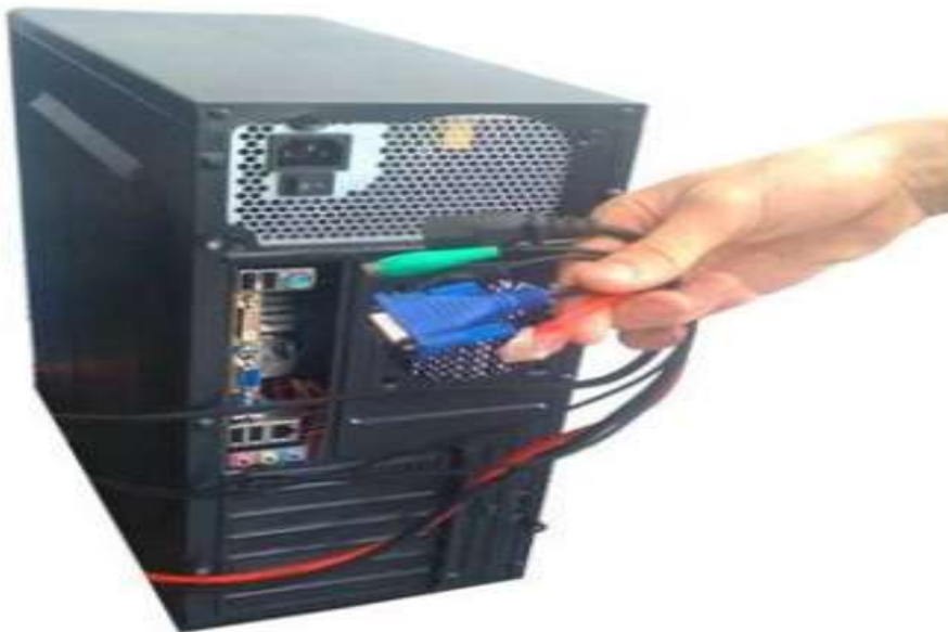
Figure 2. Disconnecting all external cables.
