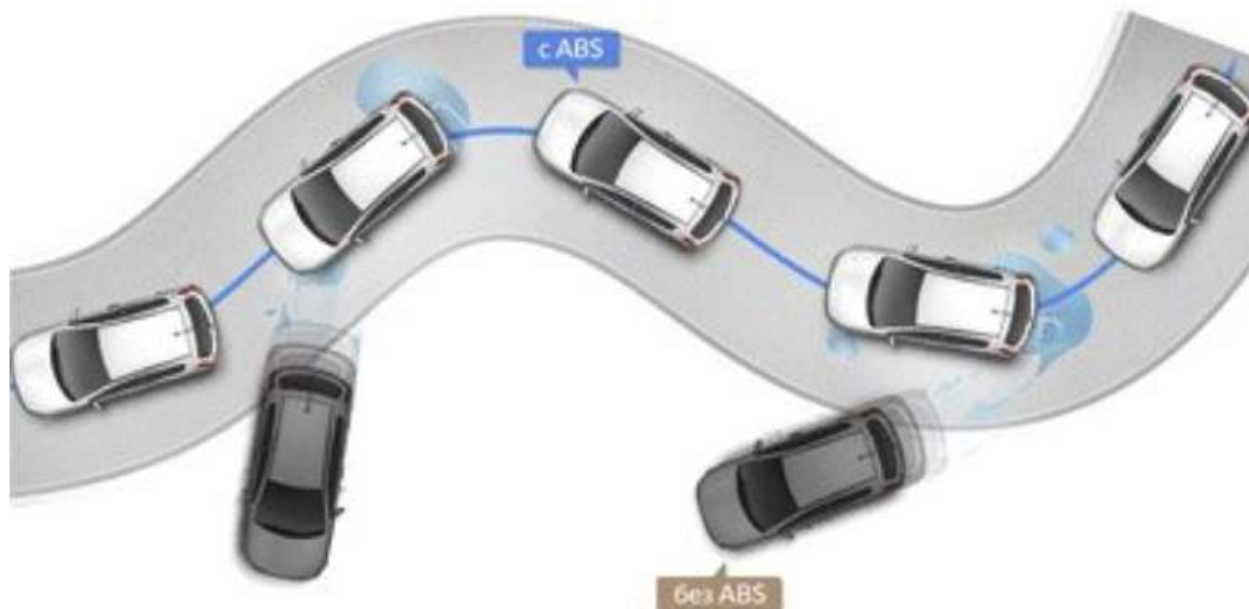
2-rasm. ABS tormoz tizimi va ABS tizimisiz harakat
