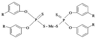
These additives are obtained by the reaction of alkylphenol with phosphorus pentasulfide and calcium salts.
