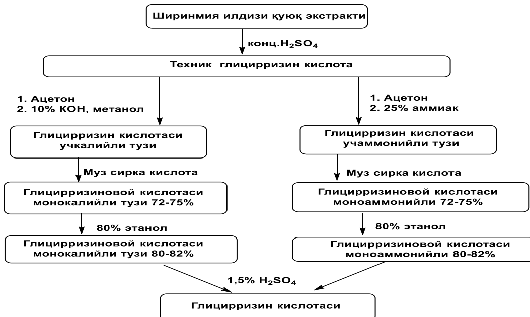
Scheme 4. Extraction of GK, GKMAT and GKMKТ from the root extract of Glycyrrhiza glabra (liquorice)
